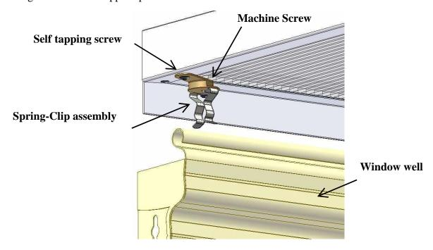
If necessary loosen the Machine screw to rotate the Spring-Clip. Caution: Loosen the screw just enough to rotate the Spring-clip!
