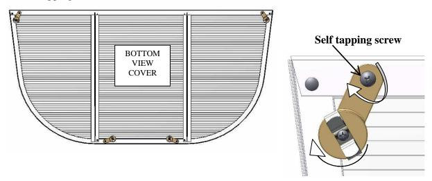
P.O. Box 250 Adel, IA 50003 (515) 993-4561 (800) 343-9370 Fax: (515) 993-4372 1850 West Adriatic Place Englewood, CO 80110 (303) 935-4679 Fax: (303 935-4670 3.) Place the Cover on top of your window well and rotate the Ties and the Spring-clips for proper alignment with the upper lip of the well.
